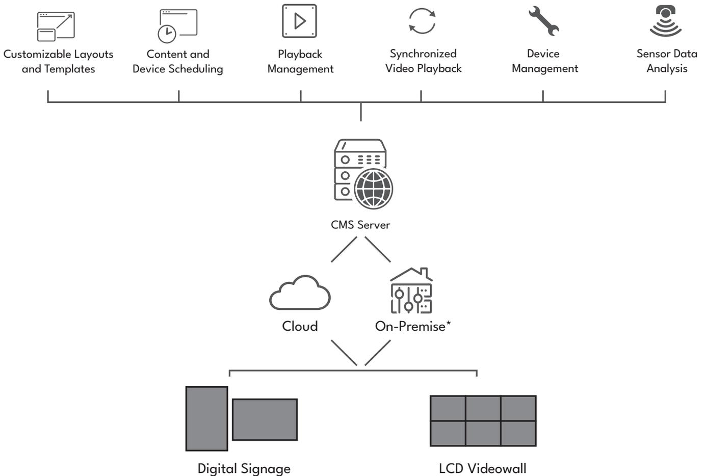
VSign is based-on three main structures which are content management, device management and sensor monitoring. The contents can be created in CMS server and sent to the displays remotely. With device management features, all Vestel displays can be controlled through Cloud or On-Premise servers. In case Vestel's Sensor Box is used with the displays, temperature, humidity, ambient light, estimated carbon dioxide, and air quality levels of the environment can be displayed in CMS server.
